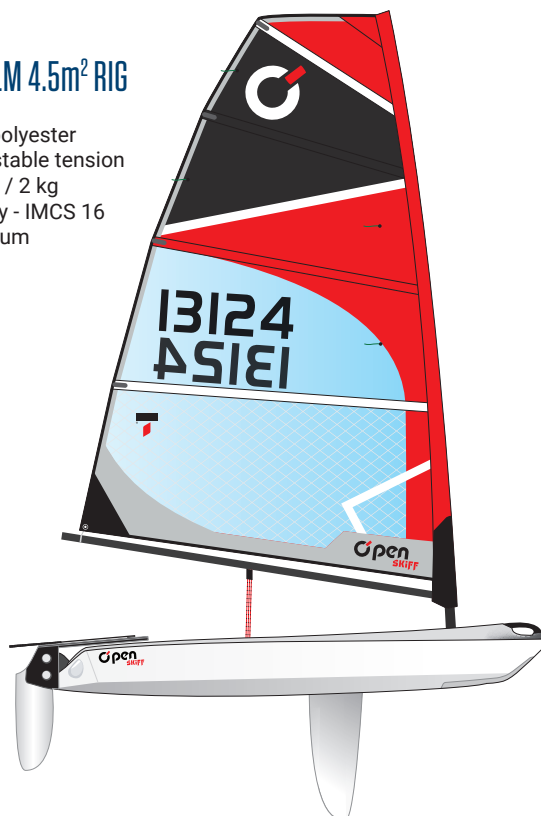
Monofilm Dacron 4.5m 2 Rig Sail: 4.5m 2 | Mast: 3.90m | Boom: 2.00m
